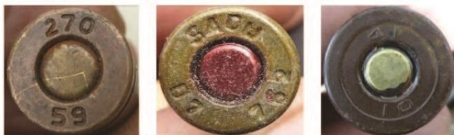
The cartridge can be pushed into soft ground or held between fingers when taking the photo. If several rounds or shells bear identical marks, a photo of one such round or shell suffices. If marks differ, photos that show marks of each round or shell with “unique” marks are required.
